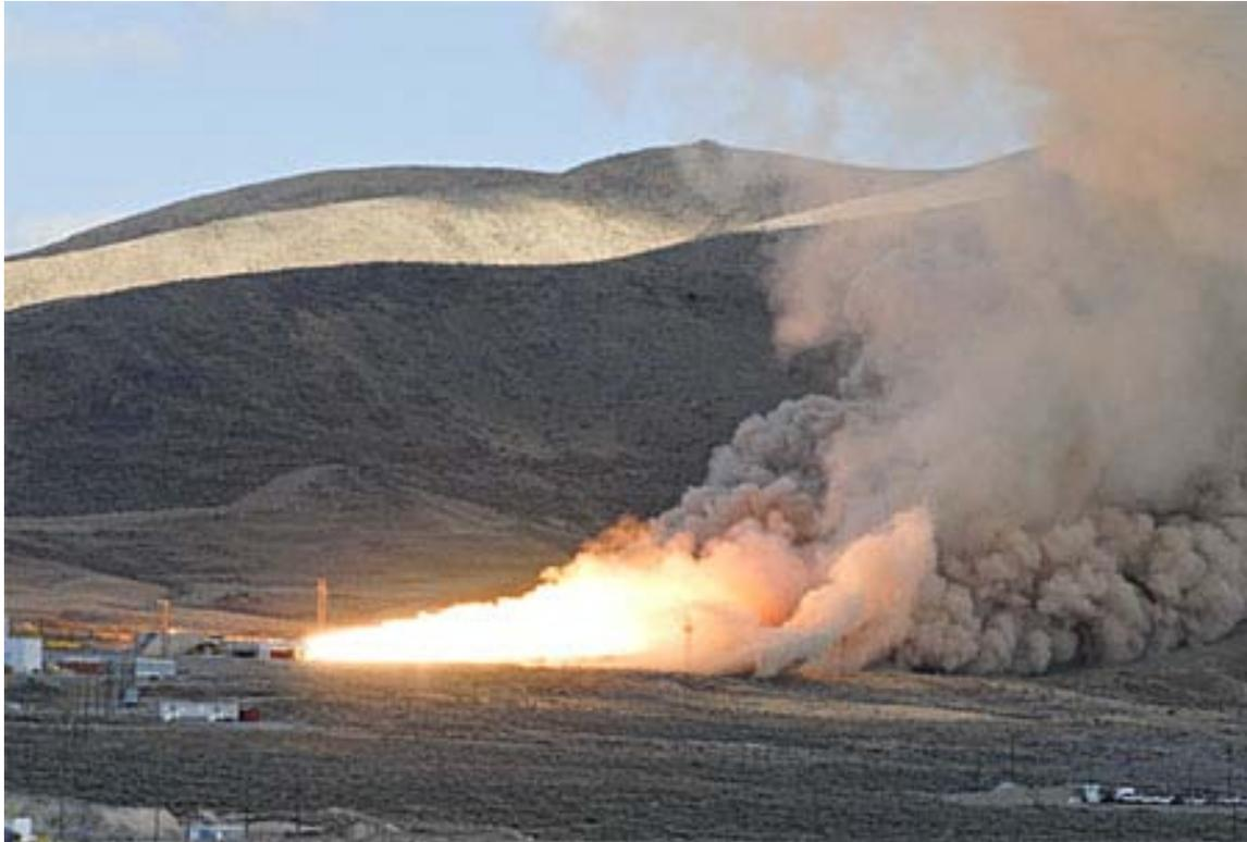
***Fire and smoke billow from a Space Shuttle solid rocket motor static test conducted in December 2008 at an ATK Launch Systems facility in Utah. These Shuttle tests have aided Ares I designers because the motors are outfitted with sensors to obtain valuable data. (ATK photo)***
