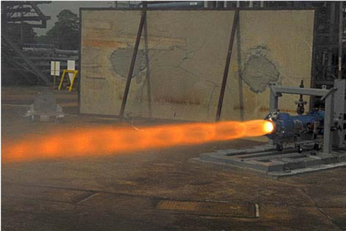
***Marshall Center engineers designed and built ullage settling motors for the Ares I upper stage. These small solids, which settle propellant so that it flows smoothly to the engine, were tested in 2008.***
