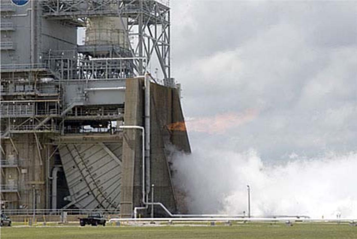
***The J-2X engine is based on the J-2 engine used by the Saturn V upper stages. The powerpack from a modified J-2 engine was used for engine performance tests. Powerpack 1A, Test 8 (shown here) ran for 324.4 seconds on April 24, 2008.***
