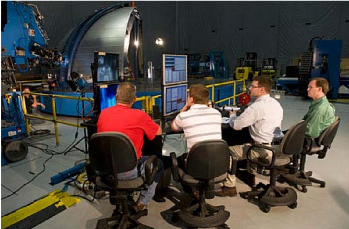
***New state-of-the-art friction stir welding machines have been installed at Marshall. Engineers are using the machines to perfect welding techniques and make a manufacturing demonstration article of the Ares I upper stage.***
