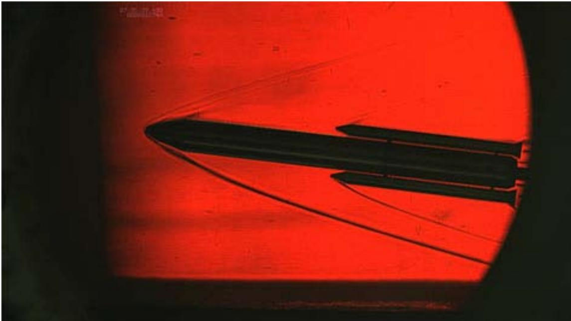
***The schlieren photo depicts one of the first Ares V wind tunnel tests at Marshall in October 2008. The photo shows airflow over a 0.35 percent model of the Ares V launch vehicle. Marshall engineers are collecting aerodynamic data to help the Ares V team determine basic requirements for guidance, navigation, and control of the huge Ares V cargo launch vehicle.***
