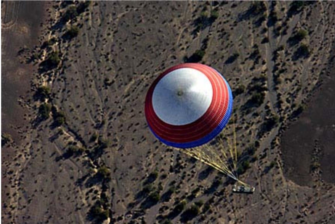
***All three types of parachutes needed to recover the Ares I first stage have undergone drop tests, such as main parachute test shown here. Tests are conducted at the U.S. Army Yuma Proving Ground in Arizona. Measuring 150-feet in diameter and weighing 200 pounds, the main parachute is the largest parachute of its kind.***
