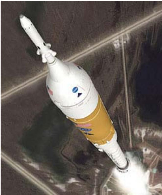
***Ares I will carry the Orion crew exploration vehicle to orbit. The Launch Abort System on top of the capsule is a crew safety feature that allows the crew to escape if there is a problem during launch.***
