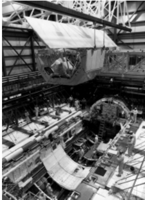
Installation of OSTA-1 in the orbiter Columbia before the second Shuttle mission in November 1981.
