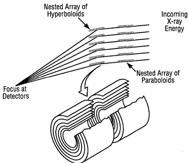
**Grazing incidence mirrors—Top illustration shows incoming x-ray energy as it is bent by the mirrors toward the focal point; bottom sketch is of nested mirror pairs.**
