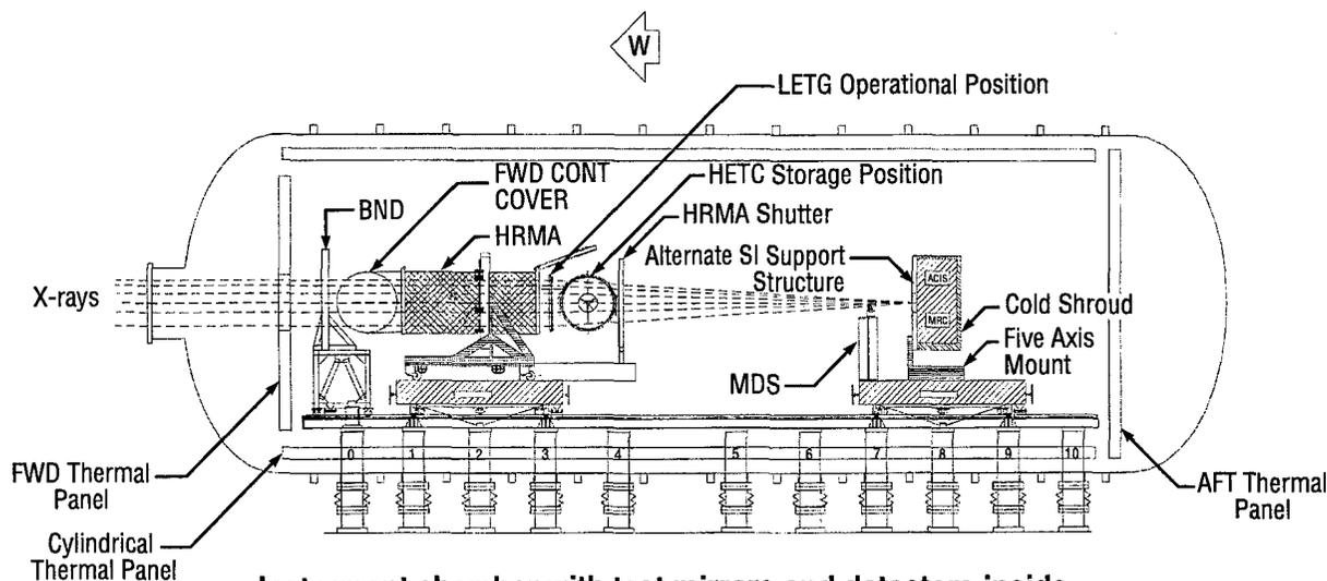
**Instrument chamber with test mirrors and detectors inside.**
