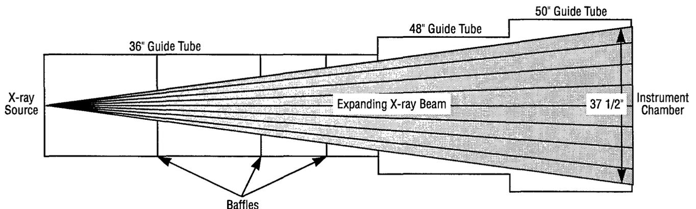
**Expanding X-ray beam as it travels through guide tube (proportions exaggerated).**
