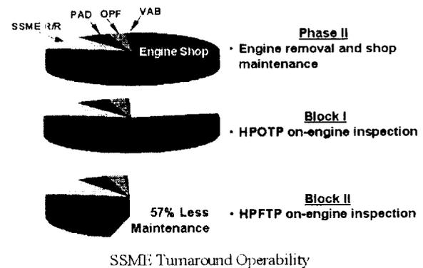
The first two single-engine flights of the Block II occurred on STS-104 and STS-109 in July 2001 and March 2002, respectively, followed by the first 3-engine cluster flight on STS-110 in April 2002. The HPFTP had accumulated 150,843 seconds of engine test maturity at the time of the first flight and is continuing a reliability demonstration test program to validate the 10 mission between overhaul goal.
